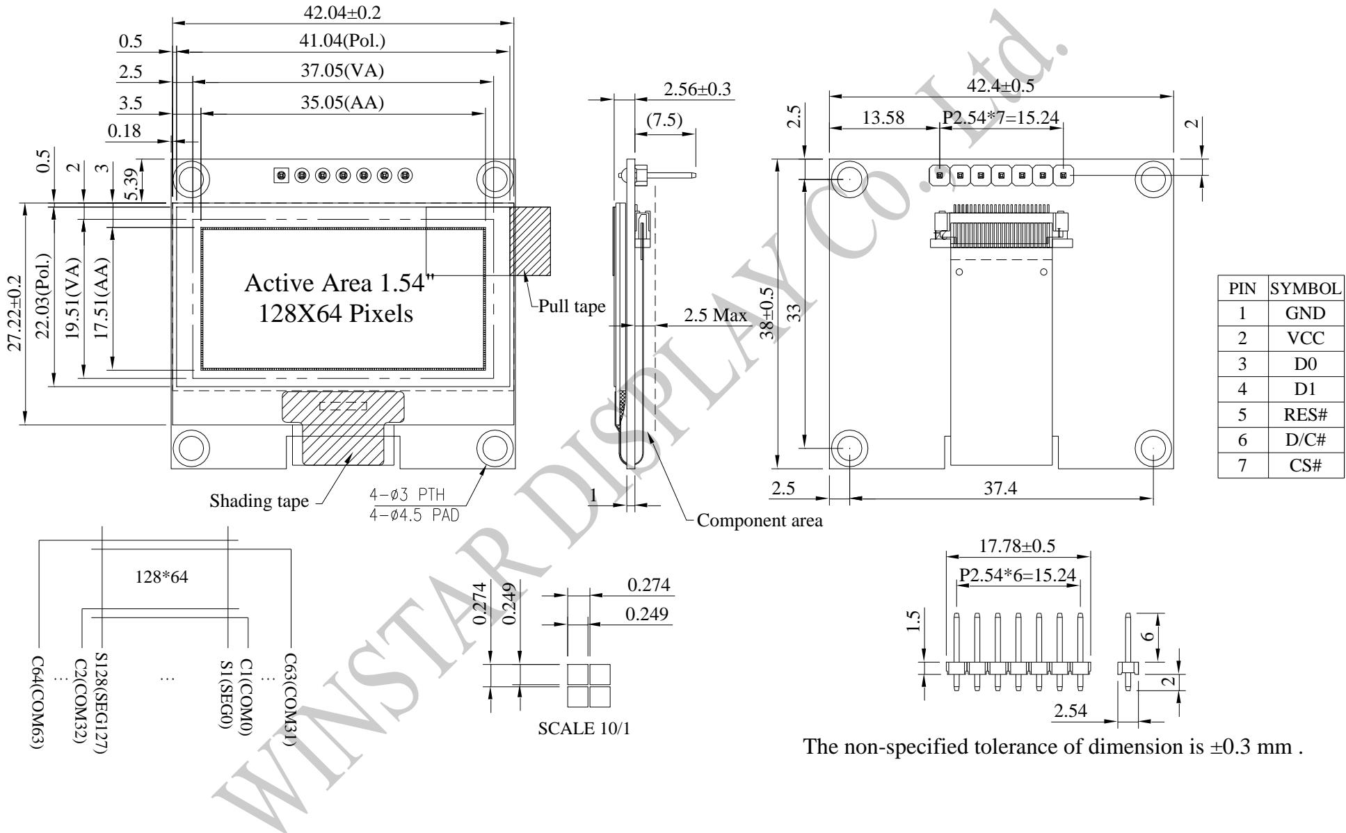
The non-specified tolerance of dimension is  $\pm 0.3$  mm.
