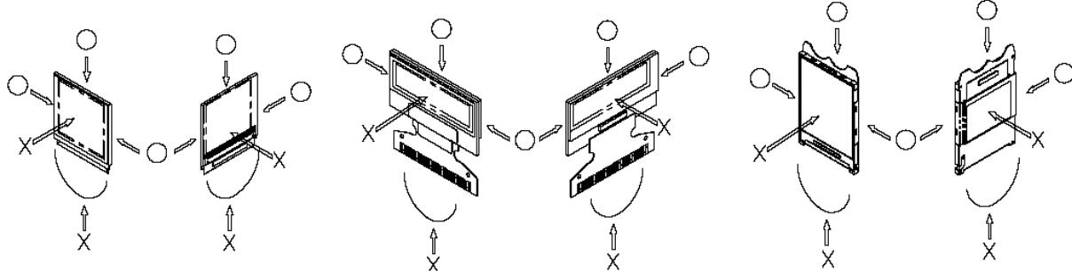
(9) Do not apply stress to the LSI chips and the surrounding molded sections.
