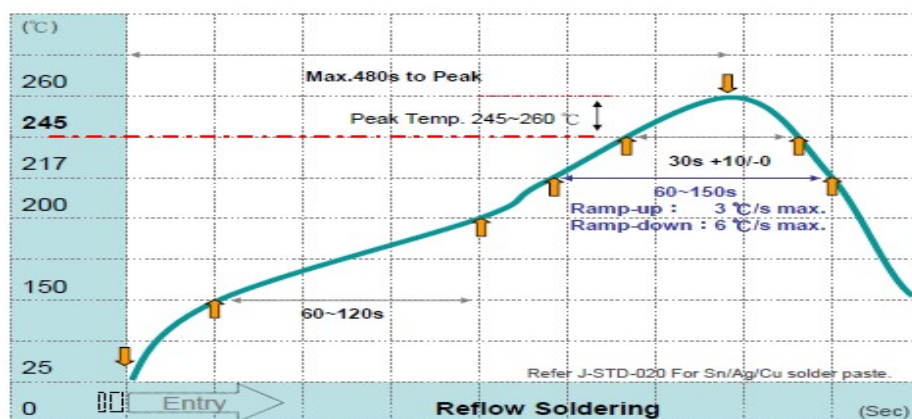
Fig 3. Infrared soldering profile for Chip Resistors WW25A
