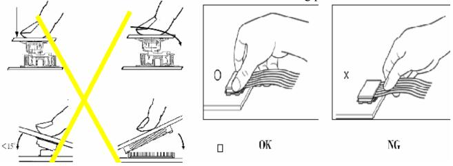
Precaution for soldering to the LCM
