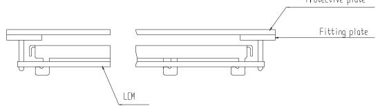
(2) When assembling the LCM into other equipment, the spacer to the bit between the LCM and the fitting plate should have enough height to avoid causing stress to the module surface, refer to the individual specifications for measurements. The measurement tolerance should be  $\pm 0.1$ mm.
