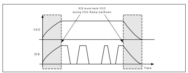
Figure 30b. Power-up, Power-Down Requirement
