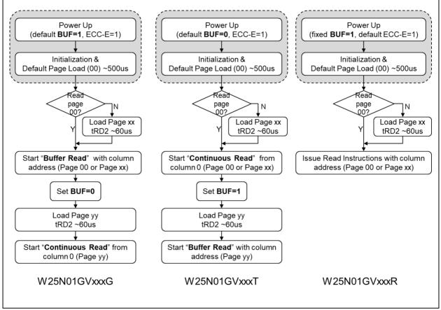
Figure 3. W25N01GV Flash Memory Operation Diagram
