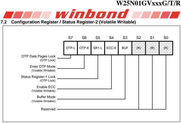
Figure 4b. Configuration Register / Status Register-2 (Address Bxh)
