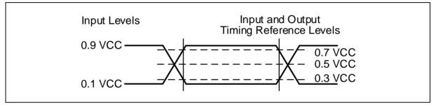
Figure 31. AC Measurement I/O Waveform
