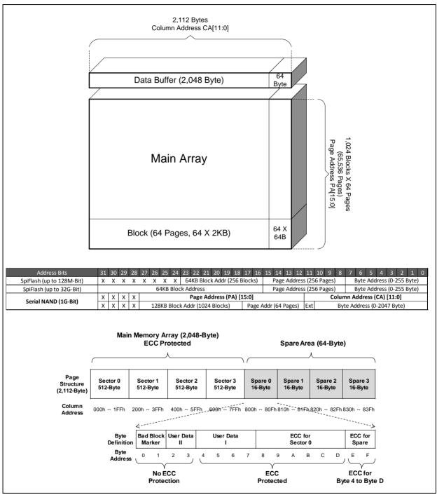
Figure 2. W25N01GV Flash Memory Architecture and Addressing
