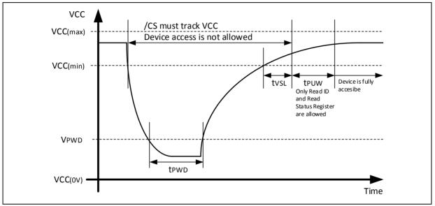
Figure 30a. Power-up Power-down Timing and Voltage Levels
