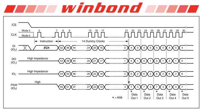
Figure 29b. Fast Read Quad I/O with 4-Byte Address Instruction (Continuous Read Mode, BUF=0)
