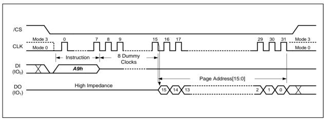
Figure 13. Last ECC Failure Page Address Instruction
