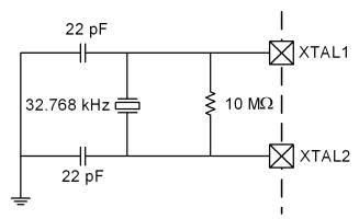
Figure 14.2. 32.768 kHz External Crystal Example
