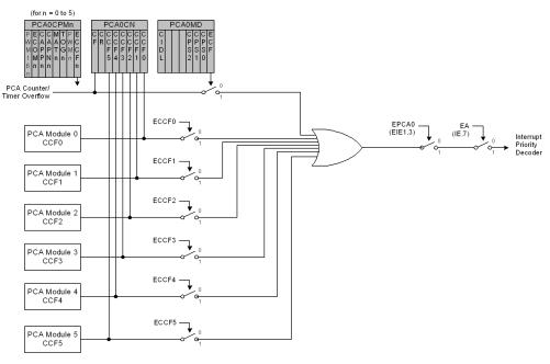
Figure 24.3. PCA Interrupt Block Diagram
