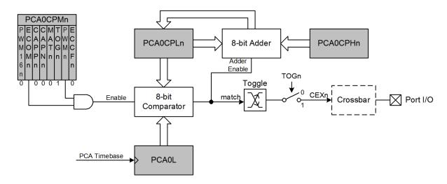
Figure 24.7. PCA Frequency Output Mode
