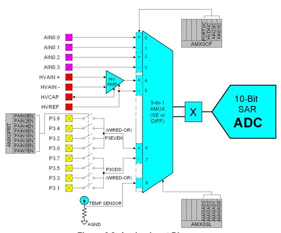
Figure 6.2. Analog Input Diagram
