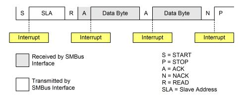
Figure 19.5. Typical Master Receiver Sequence
