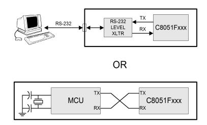
Figure 22.3. UART Interconnect Diagram
