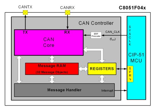
Figure 18.2. CAN Controller Diagram
