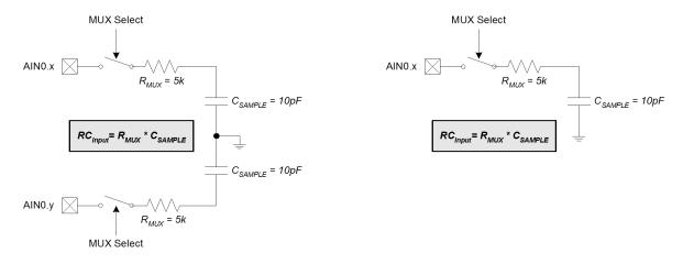
Figure 6.5. ADC0 Equivalent Input Circuits
