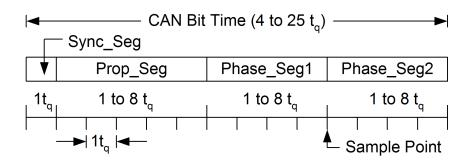
Figure 18.3. Four Segments of a CAN Bit Time
