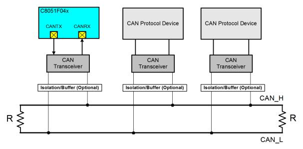
Figure 18.1. Typical CAN Bus Configuration
