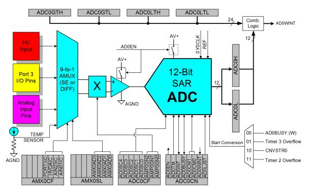
Figure 5.1. 12-Bit ADC0 Functional Block Diagram
