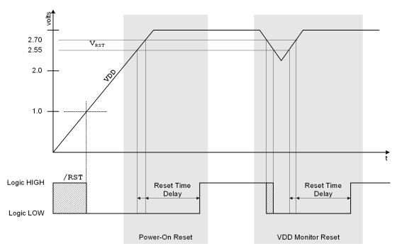
Figure 13.2. Reset Timing
