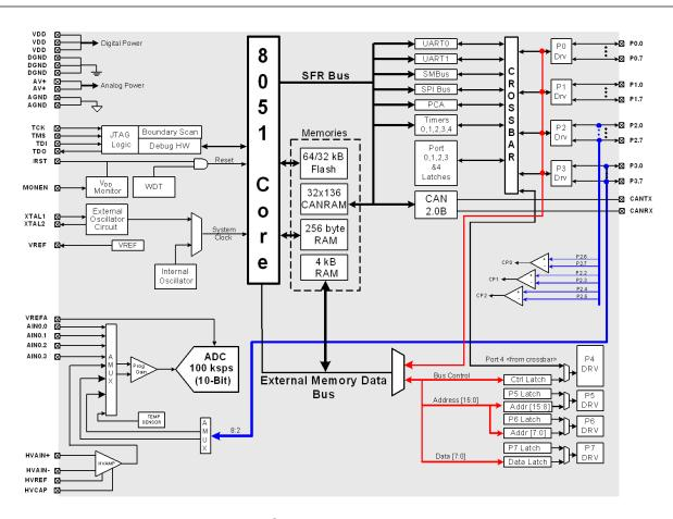
Figure 1.4. C8051F045/7 Block Diagram
