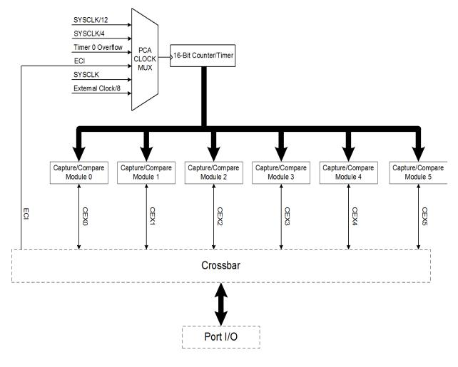
Figure 24.1. PCA Block Diagram
