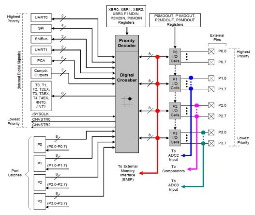
Figure 17.2. Port I/O Functional Block Diagram
