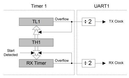
Figure 22.2. UART1 Baud Rate Logic
