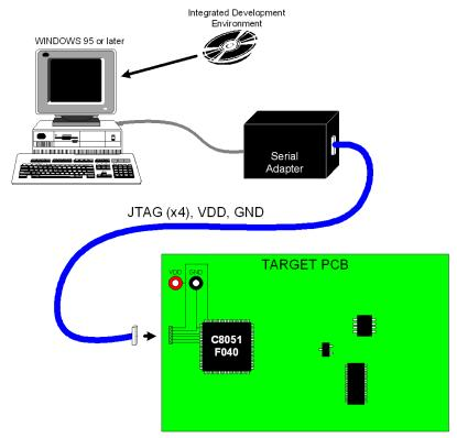
Figure 1.8. Development/In-System Debug Diagram
