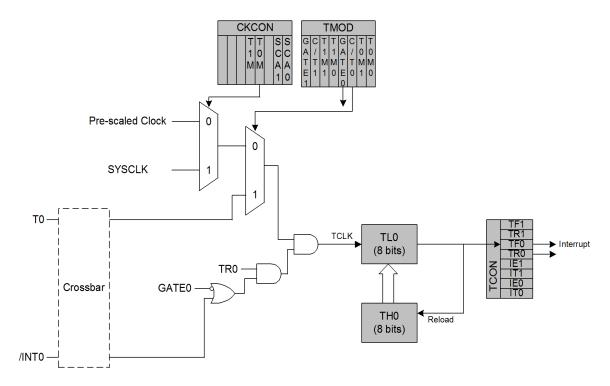
Figure 23.2. T0 Mode 2 Block Diagram
