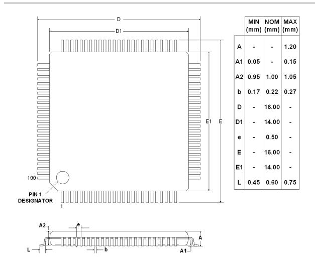
Figure 4.2. TQFP-100 Package Drawing
