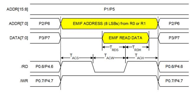
Figure 16.5. Non-multiplexed 8-bit MOVX without Bank Select Timing
