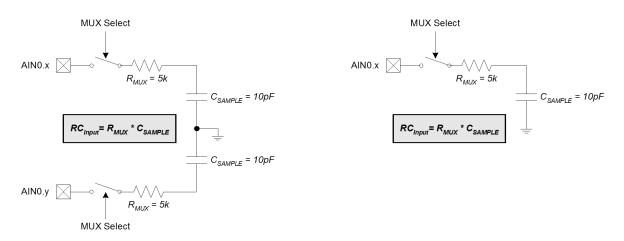
Figure 5.5. ADC0 Equivalent Input Circuits
