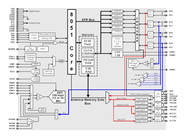
Figure 1.1. C8051F040/2 Block Diagram
