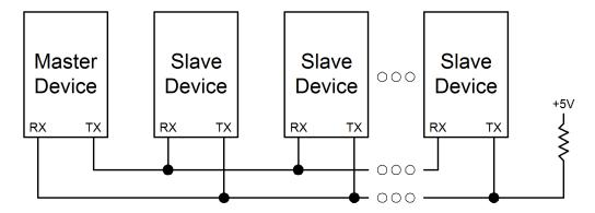
Figure 22.6. UART Multi-Processor Mode Interconnect Diagram
