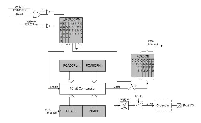
Figure 24.6. PCA High-Speed Output Mode Diagram
