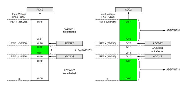
Figure 7.5. ADC Window Compare Examples, Single-Ended Mode
