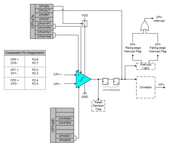
Figure 11.1. Comparator Functional Block Diagram
