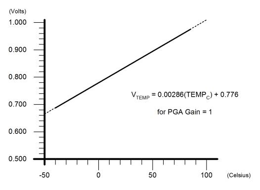
**Figure 6.6. Temperature Sensor Transfer Function**
