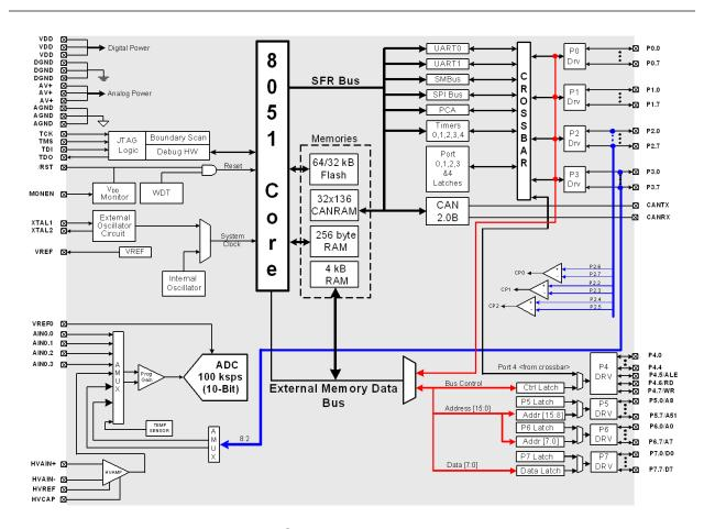
Figure 1.3. C8051F044/6 Block Diagram
