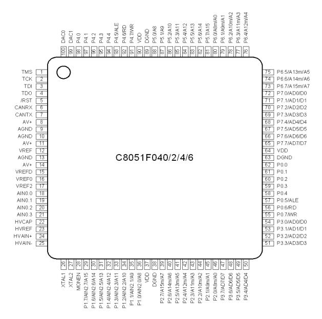
Figure 4.1. TQFP-100 Pinout Diagram
