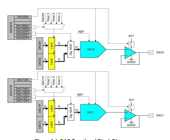
Figure 8.1. DAC Functional Block Diagram
