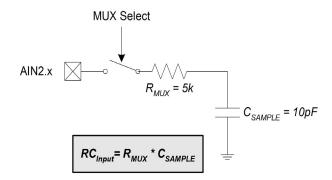
Figure 7.3. ADC2 Equivalent Input Circuit
