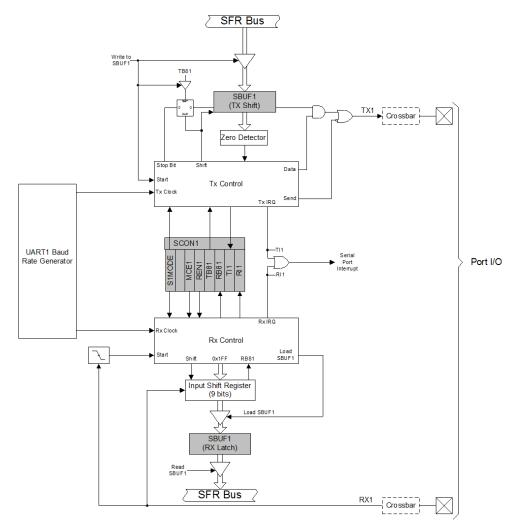
Figure 22.1. UART1 Block Diagram
