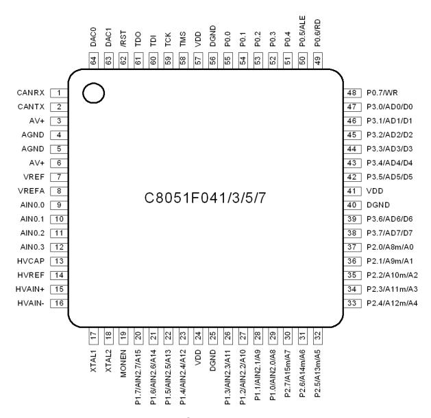
Figure 4.3. TQFP-64 Pinout Diagram
