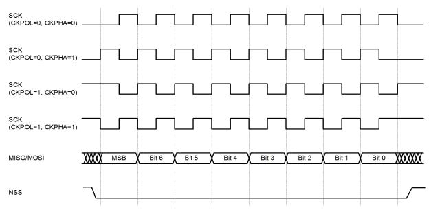
Figure 20.5. Data/Clock Timing Diagram
