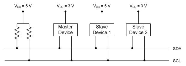
Figure 19.2. Typical SMBus Configuration
