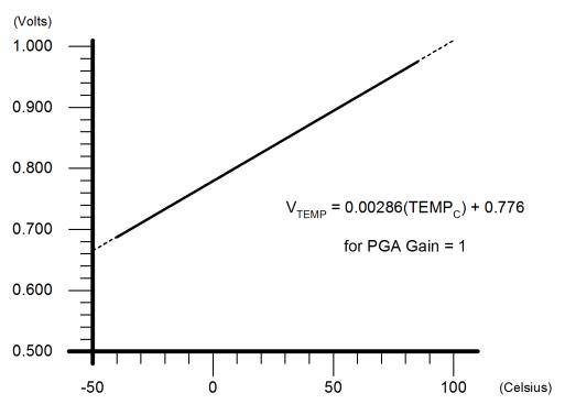
**Figure 5.6. Temperature Sensor Transfer Function**
