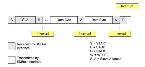
Figure 19.6. Typical Slave Transmitter Sequence
