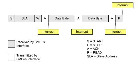
Figure 19.7. Typical Slave Receiver Sequence
