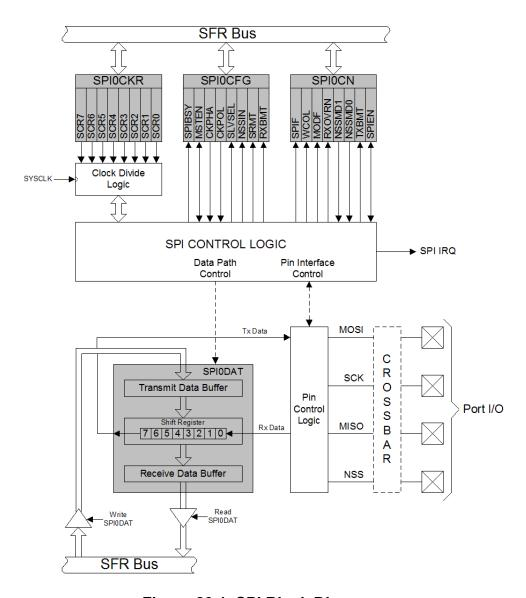
Figure 20.1. SPI Block Diagram
