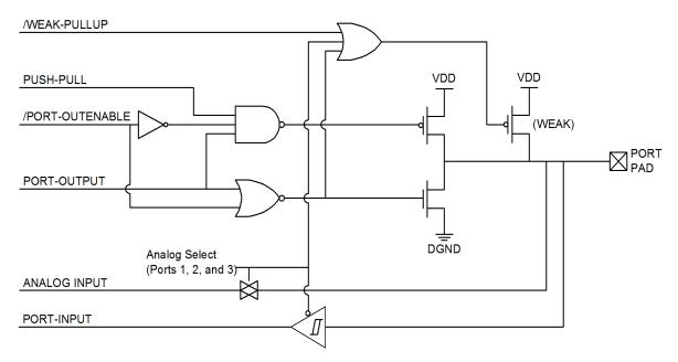
Figure 17.1. Port I/O Cell Block Diagram
