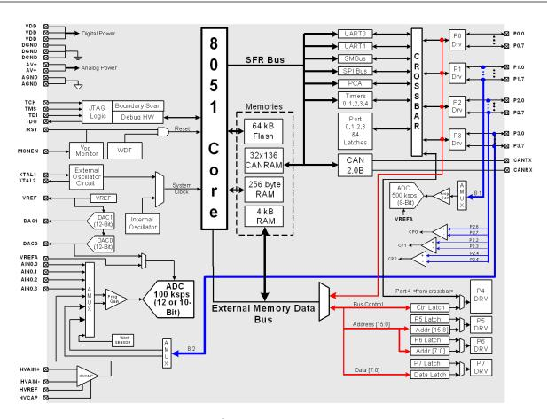
Figure 1.2. C8051F041/3 Block Diagram
