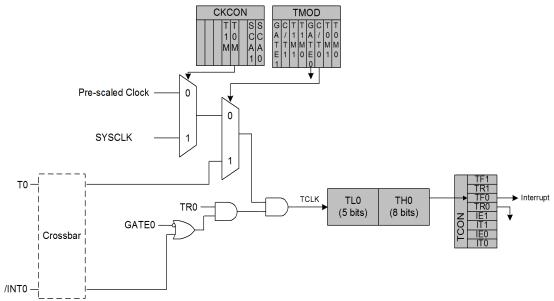
Figure 23.1. T0 Mode 0 Block Diagram
