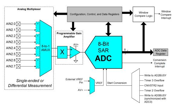
Figure 1.13. 8-Bit ADC Diagram
