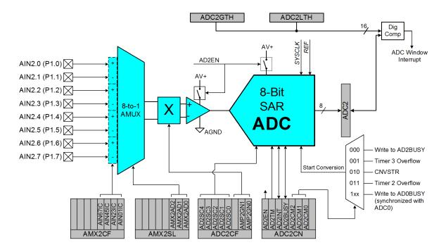
Figure 7.1. ADC2 Functional Block Diagram
