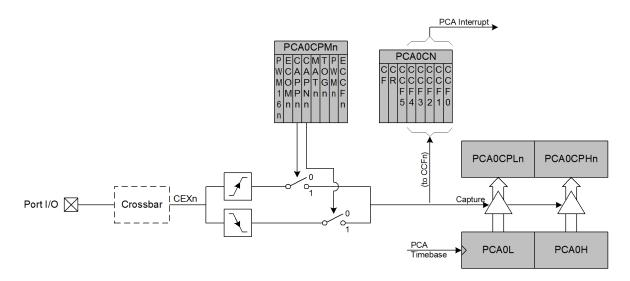
Figure 24.4. PCA Capture Mode Diagram
