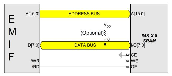
Figure 16.2. Non-multiplexed Configuration Example
