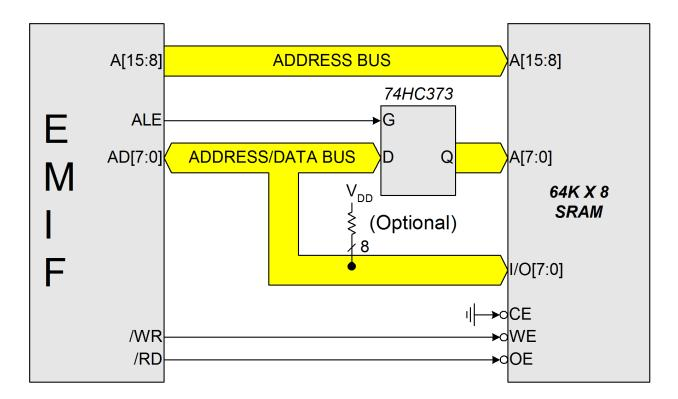
Figure 16.1. Multiplexed Configuration Example
