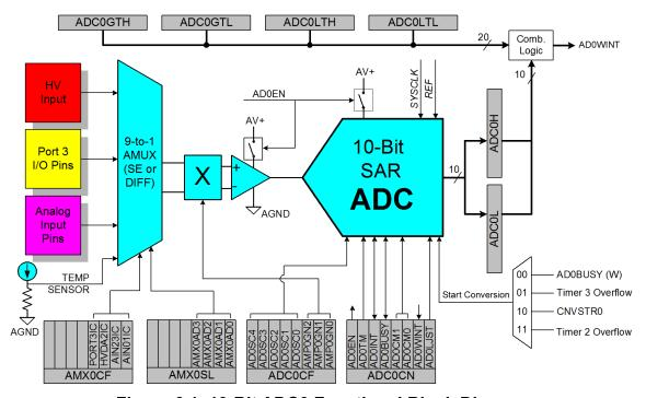
Figure 6.1. 10-Bit ADC0 Functional Block Diagram
