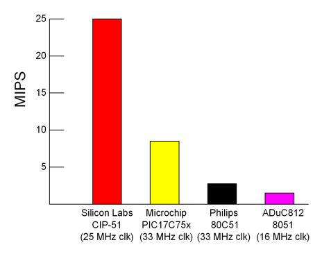
Figure 1.5. Comparison of Peak MCU Execution Speeds
