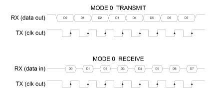
Figure 21.2. UART0 Mode 0 Timing Diagram
