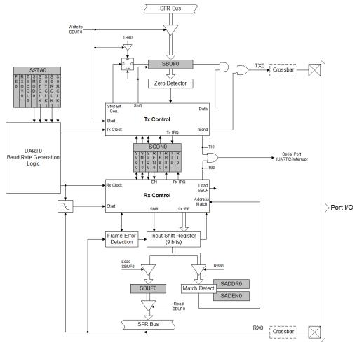
Figure 21.1. UART0 Block Diagram
