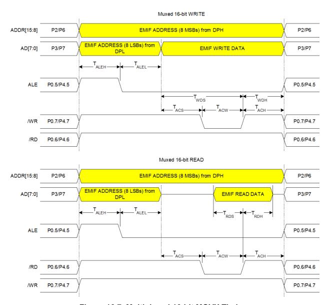
Figure 16.7. Multiplexed 16-bit MOVX Timing
