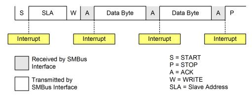
Figure 19.4. Typical Master Transmitter Sequence
