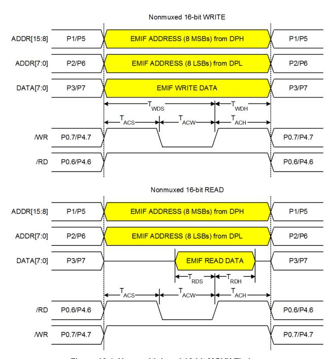
Figure 16.4. Non-multiplexed 16-bit MOVX Timing
