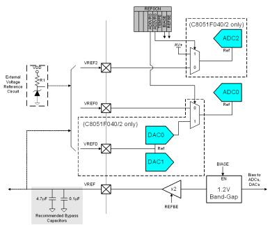
Figure 9.1. Voltage Reference Functional Block Diagram
