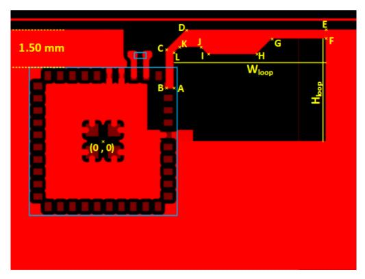
Figure 7.2. Antenna Layout With Coordinates
