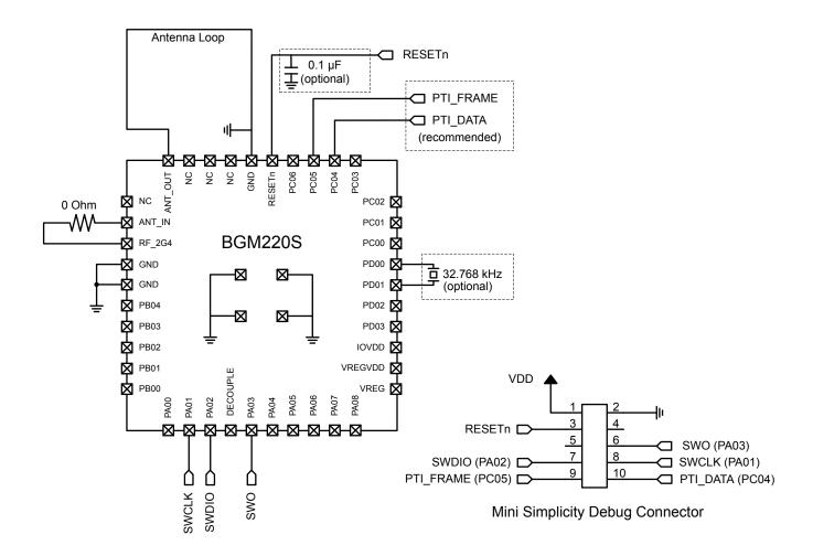
Figure 5.2. Stand-Alone SoC Configuration
