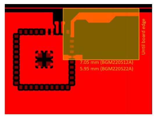
Figure 7.3. Antenna Clearance in Inner and Bottom Layers
