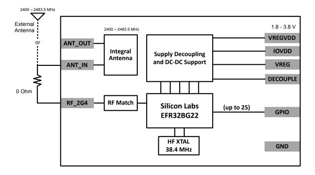
Figure 3.1. BGM220S Block Diagram
