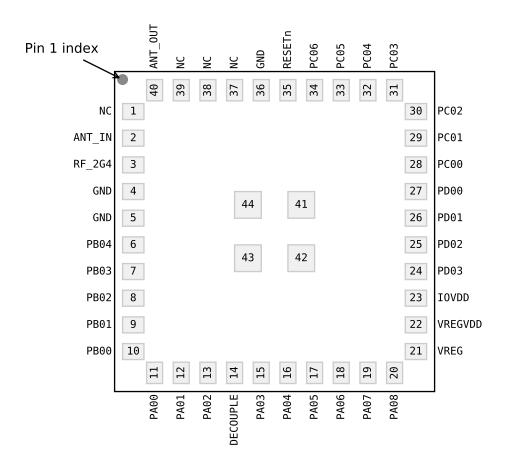
Figure 6.1. 44-Pin SiP Module Device Pinout
