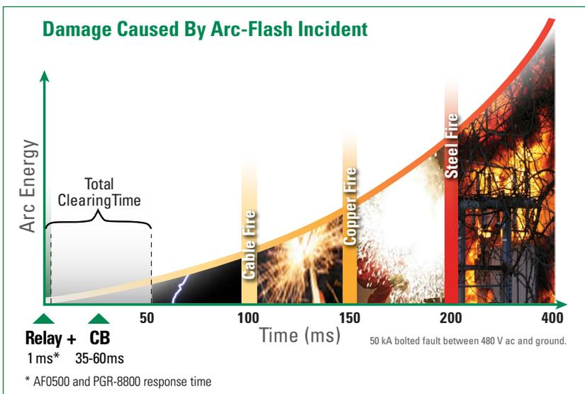
The Littelfuse Arc-Flash Relays use a 125- $\mu$ s light-sampling scheme in combination with an ultra-fast IGBT output to be able to detect a developing arc flash and send a trip signal to a circuit breaker in milliseconds.
