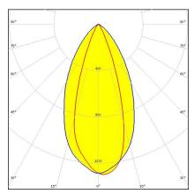
Dimensions: 21.6 mm x 21.6 mm Height: 12.85 mm ~35° + 55° rectangular beam
