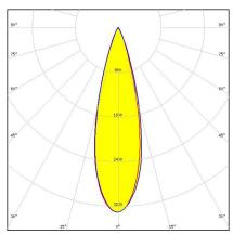
Dimensions: 21.6 mm x 21.6 mm Height: 11.90 mm ~25° medium beam
