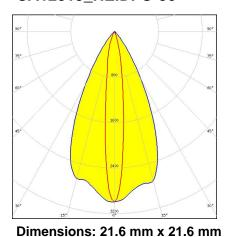
**Height: 11.70 mm** ~13° x 45° oval beam optimized for Luxeon Rebel. Variant with beam direction rotated 90°.
