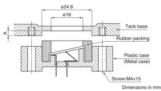
The transducer can beak off if the A dimension depth is shallow. TDK recommends a 2mm A-dimension depth and a screw tightening torque of  $0.39N \cdot m$ .
