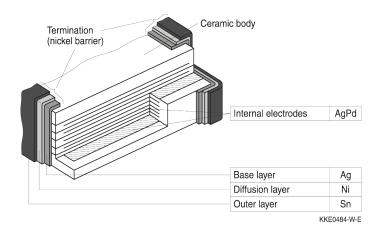
Multilayer CTVS: Structure of nickel barrier termination
