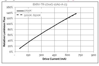
Figure 4: Relative Flux vs. Drive Current, T\_=25°C
