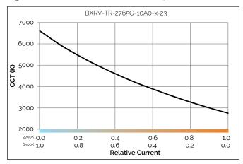
Figure 15: CCT vs. Relative Current, Tc=85C
