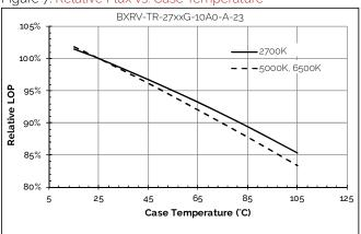
Figure 8: Relative Flux vs. Case Temperature
