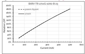
Figure 5: Relative Flux vs. Drive Current, T\_=25°C
