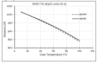
Figure 10: Relative Flux vs. Case Temperature
