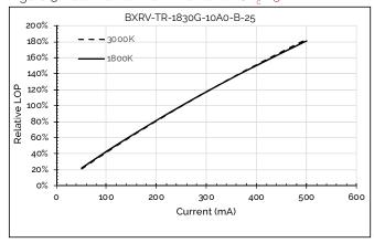
Figure 6: Relative Flux vs. Drive Current,  $T_c$ =25 $^{\circ}$ C
