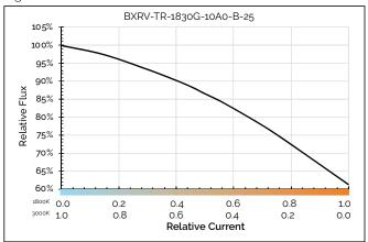
Figure 23: Relative Flux vs. Relative Current
