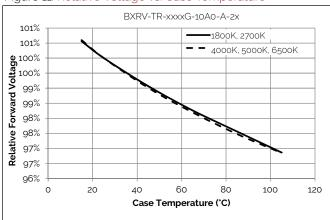
Figure 12: Relative Voltage vs. Case Temperature
