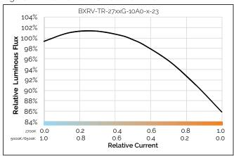
Figure 22: Relative Flux vs. Relative Current
