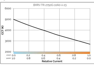
Figure 14: CCT vs. Relative Current, Tc=85C
