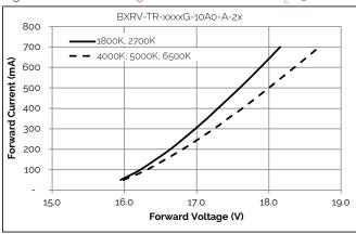
Figure 2: Forward Voltage vs. Forward Current, T\_=25°C
