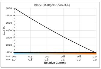
Figure 16: CCT vs. Relative Current, Tc=85C
