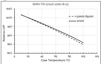
Figure 9: Relative Flux vs. Case Temperature
