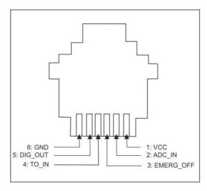
Figure 4: RJ11 Pin Connector
