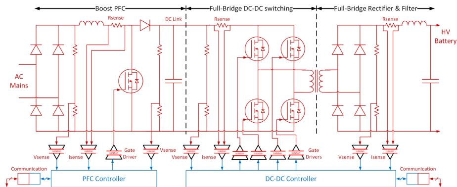
The OBC system takes the AC input source, converts it to high voltage DC through the rectifier and provides Power Factor Correction (PFC). The resulting DC signal is chopped into a switched square wave to drive a transformer to create the required output DC voltage. The chopping of the input signal is accomplished using isolated gate drivers like the [Si8239x](#), [Si823x](#), [Si823Hx](#), and [Si827x](#).
