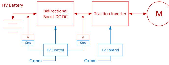
Getting optimal efficiency from the system may require peak ac voltages that exceed the vehicle's HV battery voltage, so the traction inverter is often preceded by a bidirectional dc-dc boost converter. This boost converter often contains 2 switches, which require isolated gate drivers. The system voltages can be sensed before the booster and traction inverter and a measurement taken with the [Si8931](#) isolated sensor ("Sns" in the diagram).
