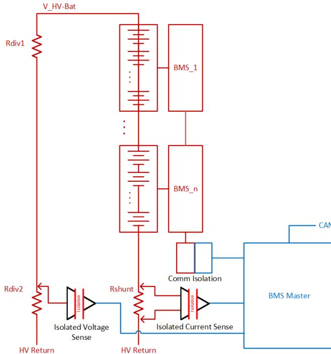
To monitor the modules and cells, the BMS may have a centralized architecture, or a distributed/modular architecture consisting of a BMS master and several remote BMS units. In distributed BMS systems, remote units monitoring individual cells may be connected in parallel to the BMS master, or they may be daisy-chained in series. In any case, connections from the battery modules or BMS remote units to the BMS master must be isolated to protect the BMS master from the battery voltages.
