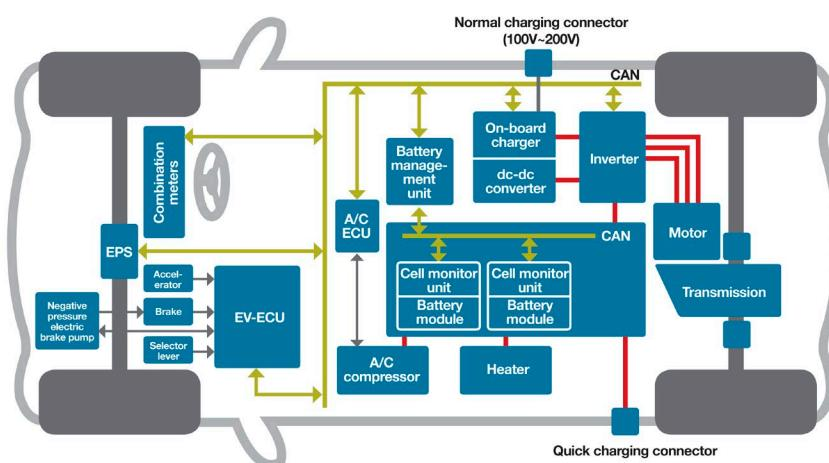
The traction inverter converts dc power from an on-board high voltage (HV) battery into ac power to drive the main motor or motors of an electric vehicle.
